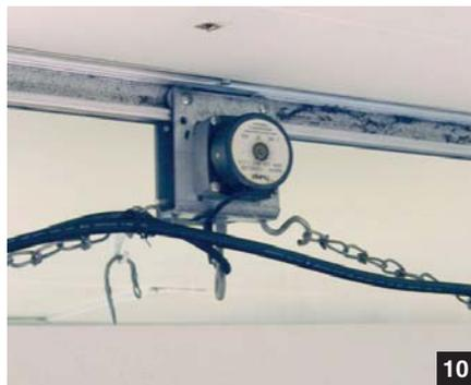
[10] A close-up view of the motorized box that attaches the HID reflector to the track on the ceiling. Small wheels attached to the motorized box roll in the bottom part of the track on the ceiling and carry the reflector back and forth across the room.
