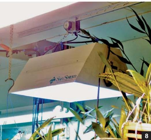
[8] An HID light reflector, with lights inside, mounted on the metal track attached to the ceiling of the room. The reflector moves back and forth across the room, driven by a motor in the small box by the mounting of the reflectors near the ceiling.
