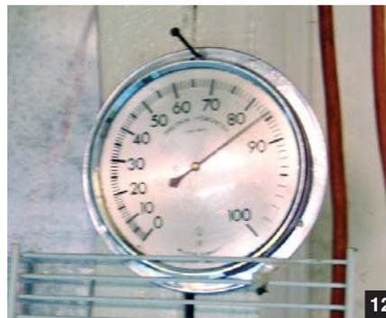
[12] A thermo-hygrometer hanging on the wall of the large intermediate room. This gauge measures temperature and humidity.
